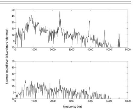
Figure 4. Spectrograms showing the scanner sound level as a function of frequency before and after cancellation.
