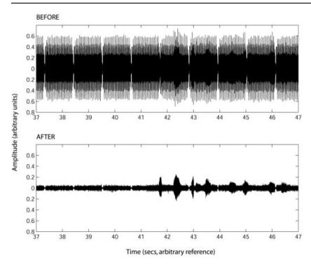
**Figure 2.** Sound waveforms before and after cancellation. After cancellation, the speech waveform is clearly visible.
